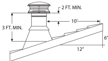
Note: The chimney must extend at least three feet above the highest point where it passes through the roof surface and at least two feet higher than any part of the building within a horizontal distance of ten feet.
