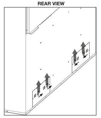
H. Rotate the blower down the side of the firebox and out of the opening. Disconnect wires.
