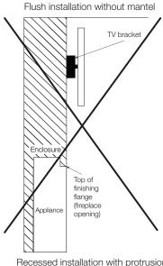
Recessed installation with protrusion
