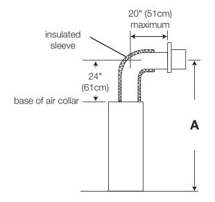
Use the periscope kit to locate the air termination above grade. The periscope must be installed so that when final grading is completed, the bottom air slot is located a minimum 12" (30.5cm) above grade. The maximum allowable vent length is 10' (3m) for a fireplace and 8' (2m) for a stove.
