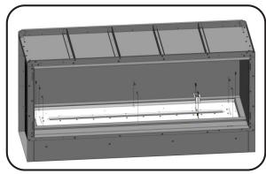
Lift the glass tray from the fireplace, pushing from the top, disengage the thermocouple and igniter from the glass tray.
