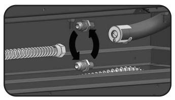
6. Replace the natural gas orifice with the LP (Propane) orifice supplied.
