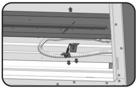
4. Disconnect the stainless steel flex connector from the orifice using (2) wrenches.
