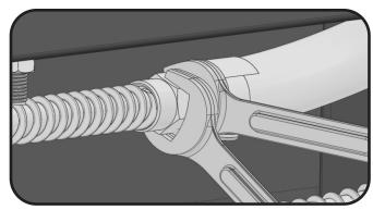
5. Unscrew the natural gas orifice from the inside of the burner as illustrated.
