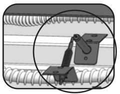
Remove the flex hose and the orifice from the burner and completely remove the glass tray from the fireplace.
