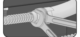
Once the glass tray is removed from the fireplace flip the glass tray upside down and remove the nuts from the bottom of the burner.
